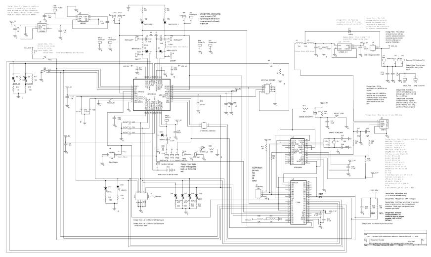
Figure 9. LP3971 Flex\_PMU Evaluation Board Schematic
