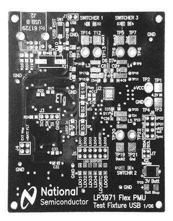
Figure 8. Bare Board/Component Locations
