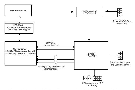
Figure 2. LP3971 Flex\_PMU USB Evaluation Board Block Operational Diagram
